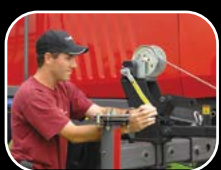
Adjustment is done manually with a winch/pulley system.
